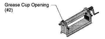
Figure 6 -- Lubricating the Gears
